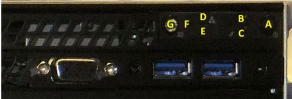
Figure 2-2: PROGUARD Status Activity LEDs, Soft Reset Button and Power Button
