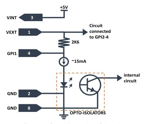
Figure 2-2: General Purpose Input Schematic
