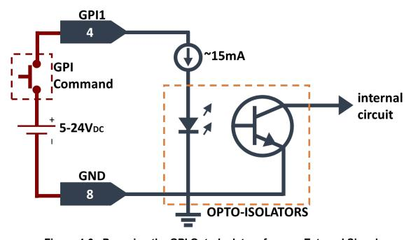
Figure 4-6: Powering the GPI Opto-Isolators from an External Signal
