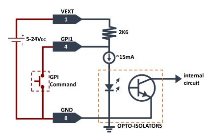
Figure 4-5: Powering the GPI Opto-Isolators from an External Power Supply
