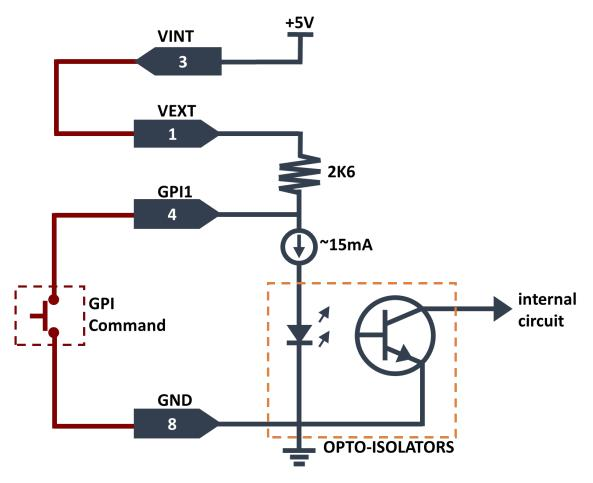
Figure 4-4: Powering the GPI Opto-Isolators from the Router
