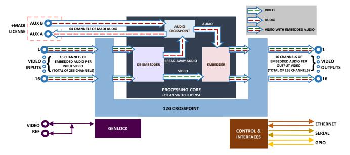
Figure 4-1: EQT Clean Switch Block Diagram
