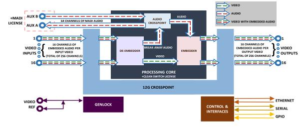
Figure 1-2 : EQT-1616-3G-F Block Diagram
