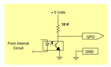
Figure 2-3: GPO Output Circuitry
