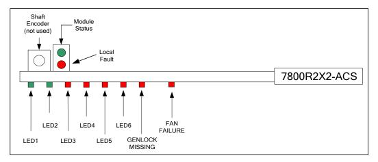
Figure 4-1: 7800R2x2-ACS-4K Status LEDs
