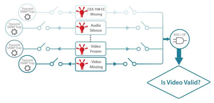
Figure 5-12: Connection Between Fault, Trap and ACS
