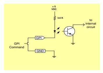
Figure 2-2 : GPI Input Circuitry
