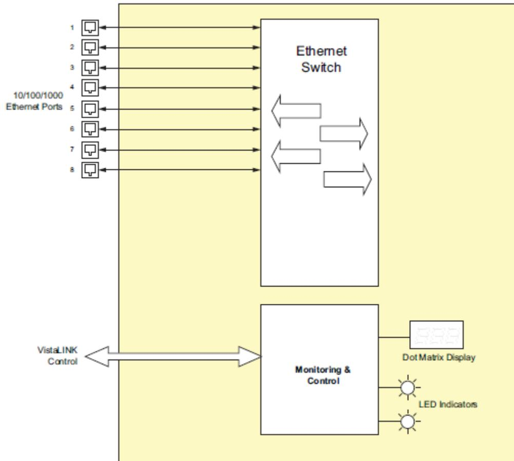
Figure 1-1 : 7880GS-8 Block Diagram
