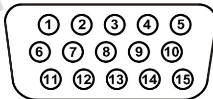
**Figure 2-4: High Density DB-15 Connector**
