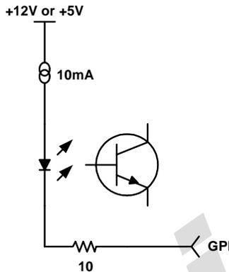
Figure 2-2: Typical GPI Circuitry
