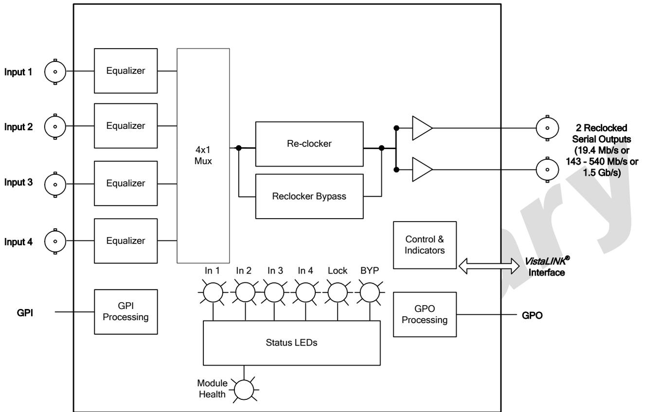
Figure 1-1: 7700R4X1-HD Block Diagram
