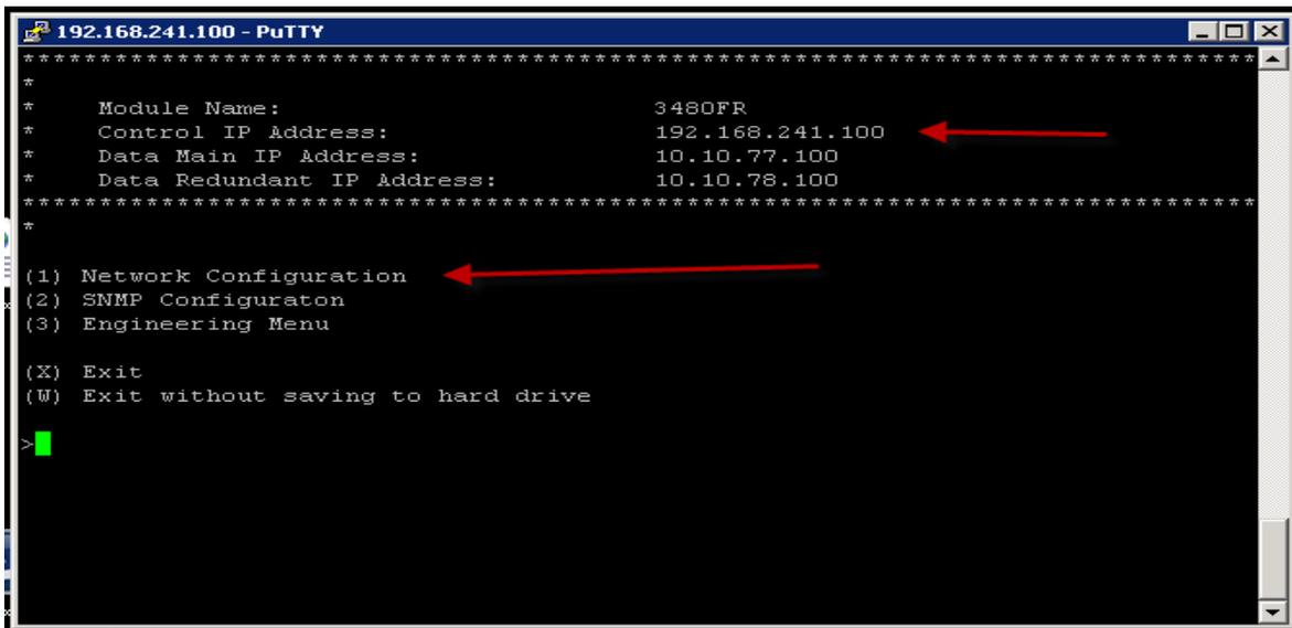
**Figure 2-3 : Configure IP Interfaces to the MUXIP**
