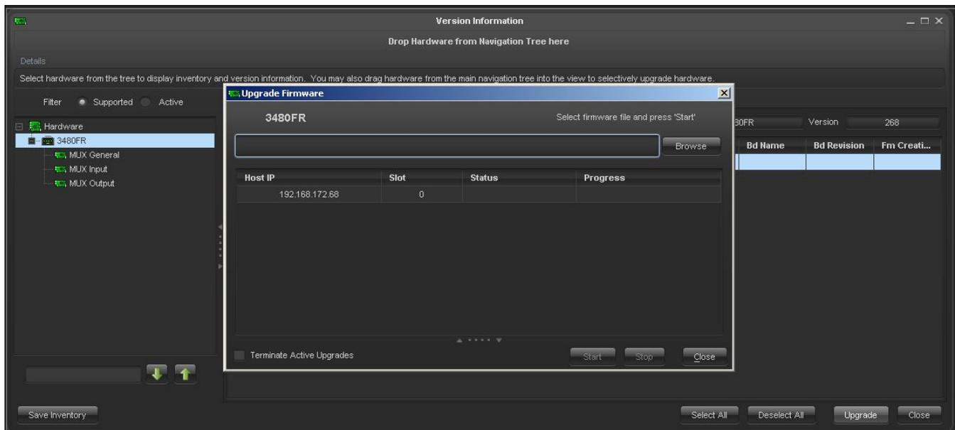
Figure 5-5 : VistaLINK® PRO – Selecting File for Firmware Upgrade
