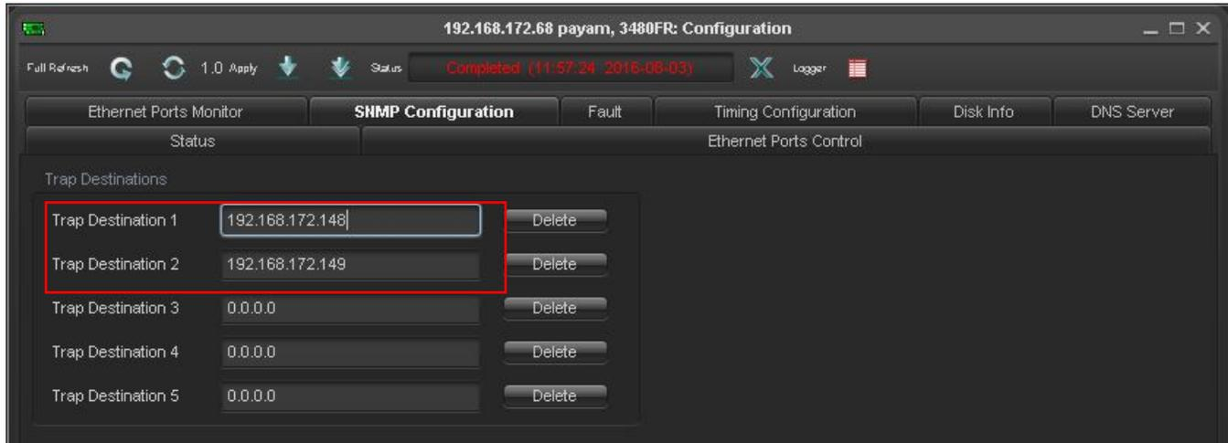
Figure 4-6 : VistaLINK® PRO Hardware Configuration - SNMP Configuration Tab
