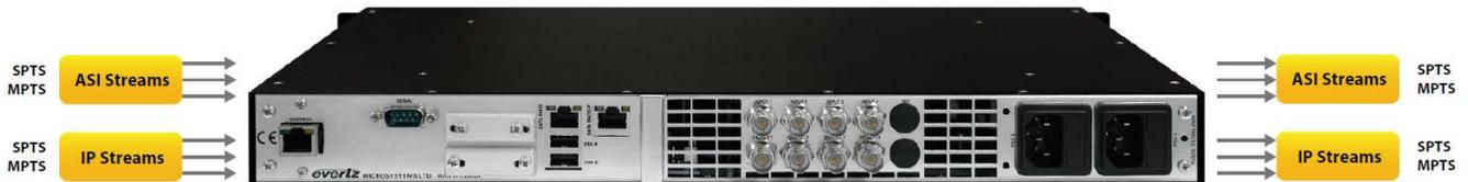
**Figure 1-2 : 9780MUX-IPGE Rear Panel**
