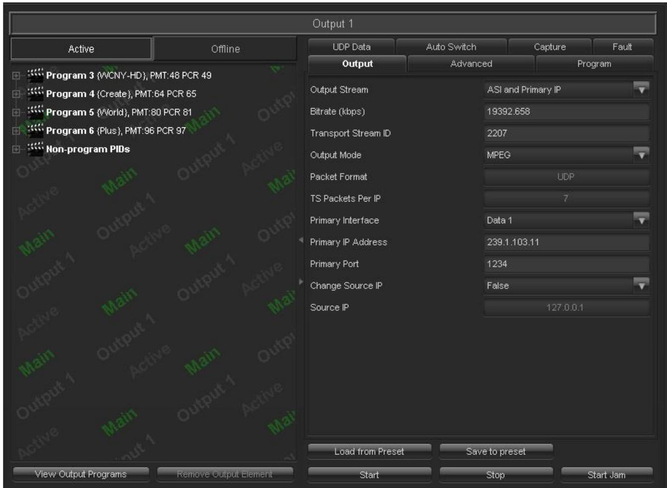
Figure 4-33 : VistaLINK<sup>®</sup> PRO – Mux Output - Output Tab
