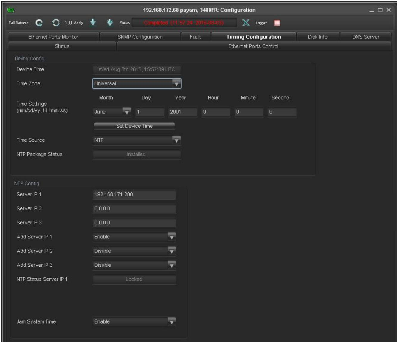
Figure 4-8 : VistaLINK® PRO Hardware Configuration – Timing Configuration Tab
