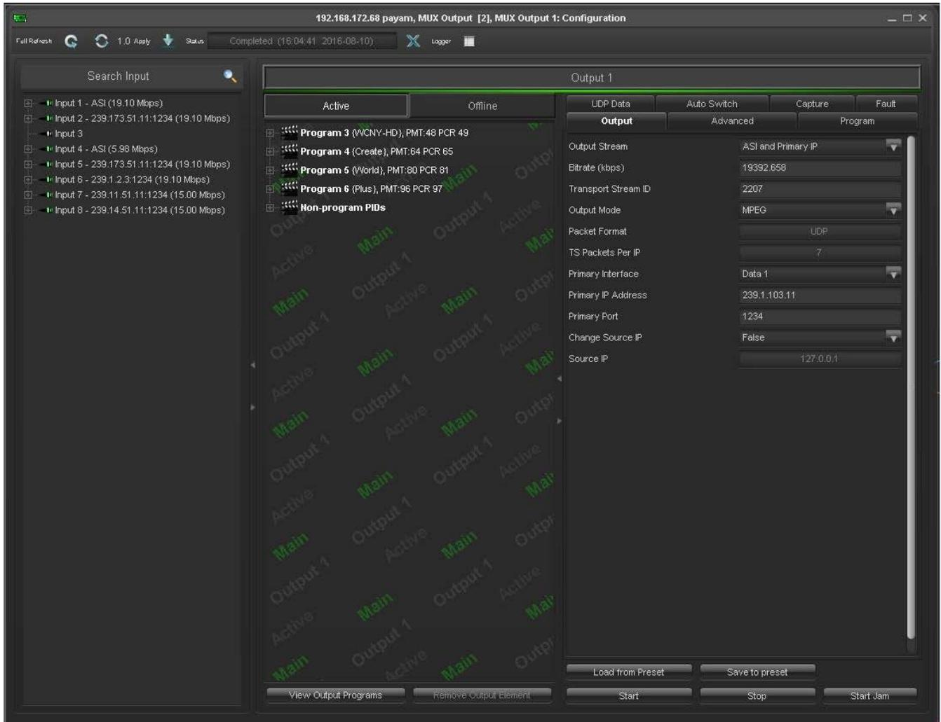
Figure 4-21 : VistaLINK® PRO - MUX Output Configuration window
