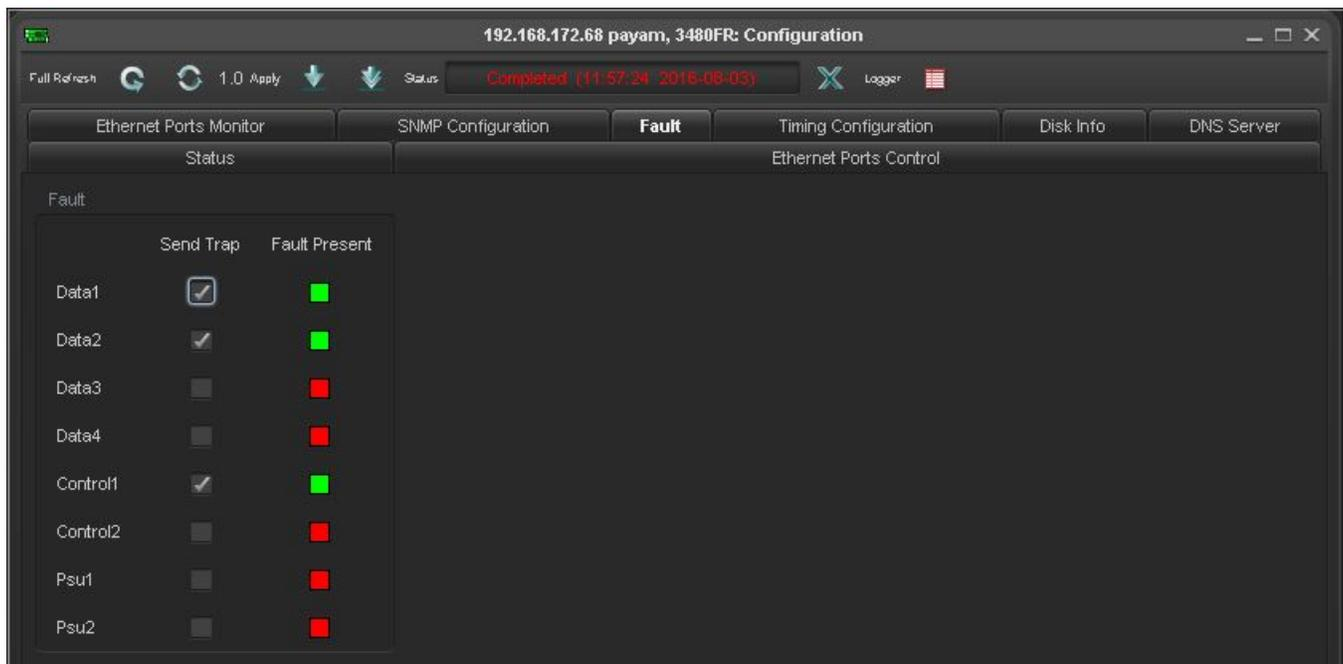
Figure 4-7 : VistaLINK® PRO Hardware Configuration - Fault Tab
