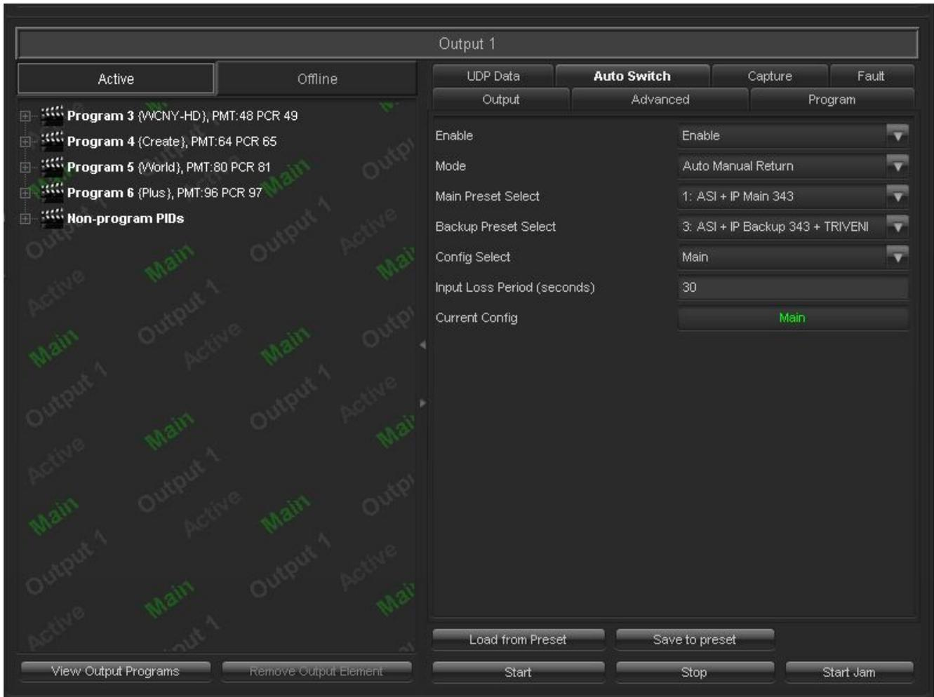
**Figure 4-37 : VistaLINK<sup>®</sup> PRO – Mux Output – Auto Switch Tab**
