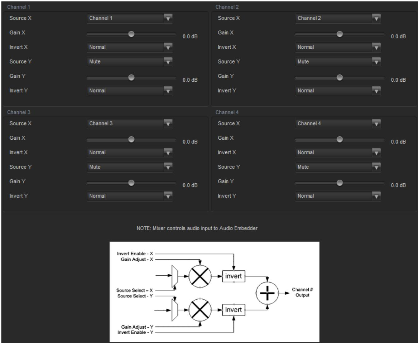
Figure 4-49: Analog Audio Mixer Tab
