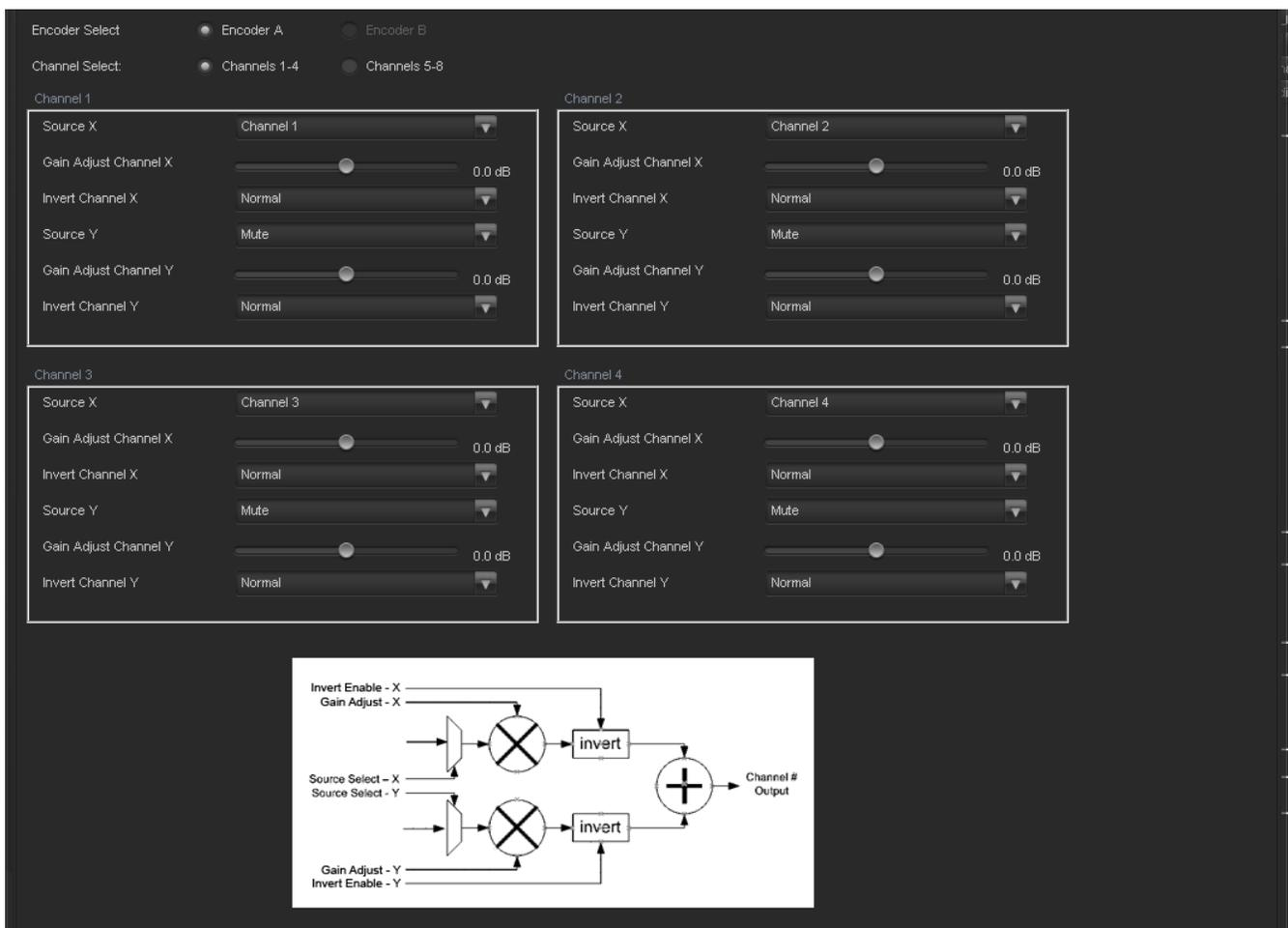
**Figure 4-42: Dolby AC3 Encoder Mixer Tab**
