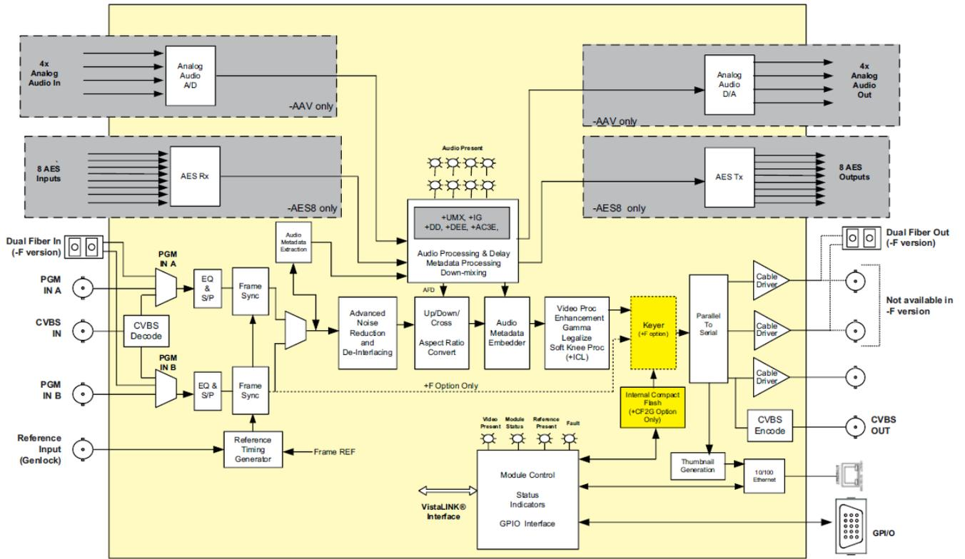
Figure 1-1: 7812UDX-AAV Block Diagram
