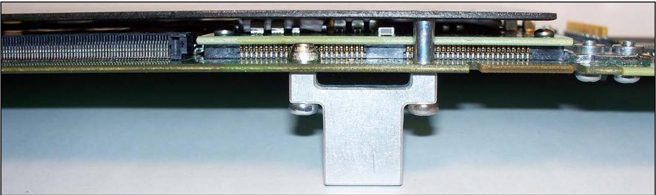
**Figure 5-3: Slot Blocker**
