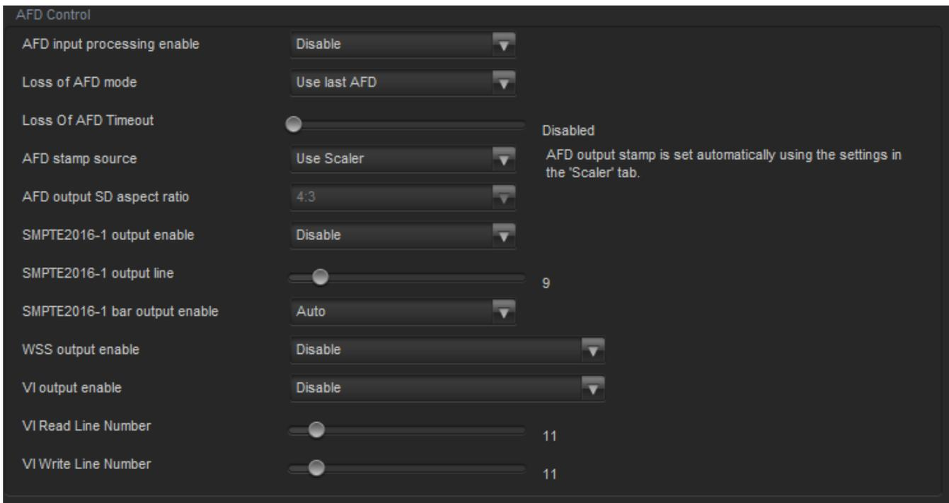
**Figure 4-19: AFD Control Tab**
