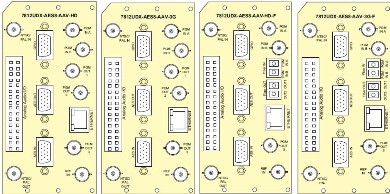
Figure 2-2: 7812UDX-AES8-AAV-xx Rear Plates
