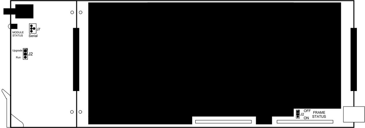
**Figure 5-1: Location of Jumpers – Top View Main Module**
