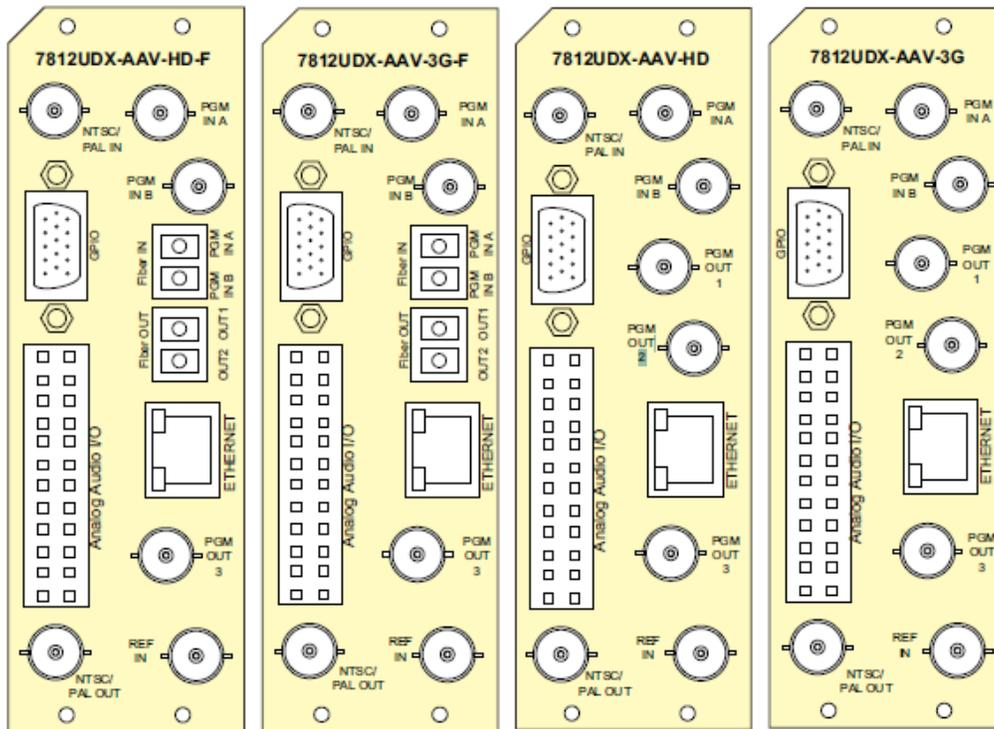
**Figure 2-1: 7812UDX-AAV-xx Rear Plates**
