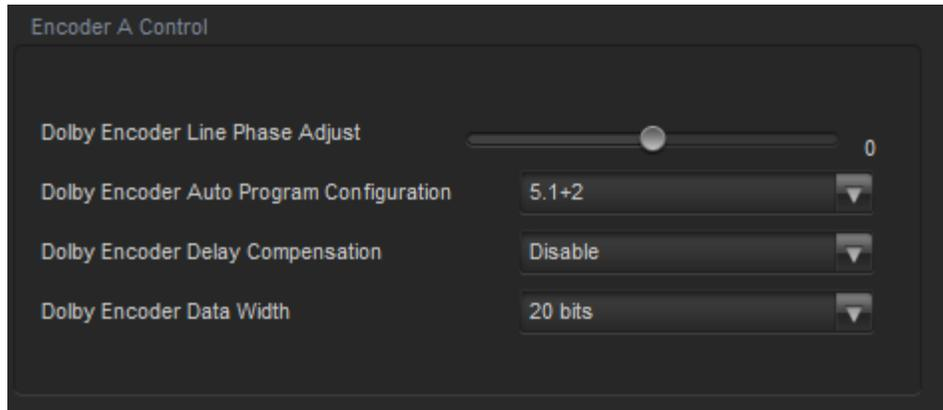
**Figure 4-39: Dolby E Encoder Control Tab**
