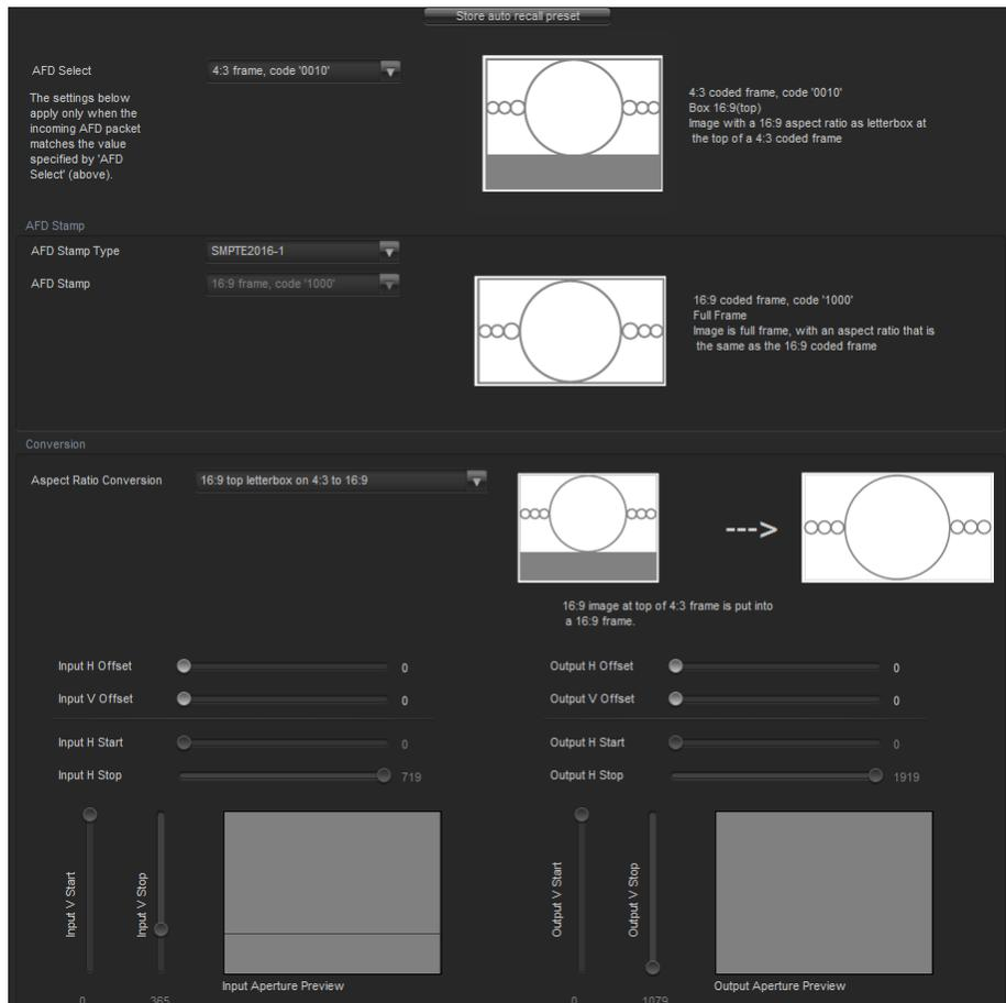
Figure 4-22: AFD ARC Tab
