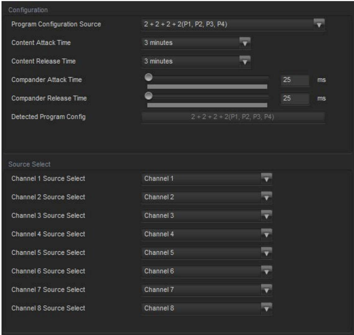
Figure 4-35: IntelliGain® Configuration Tab
