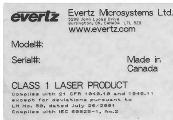
Figure 2-3: Reproduction of 7807LT-2 Certification and Identification Label for Models that are Class 1 Laser Products
