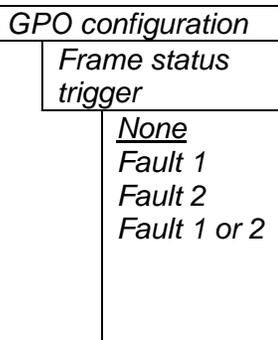
The 7700 frame has a global status line that any card can pull active. With this control, you can select the condition for the card to cause the line to go active. Also included on the frame status signal is card power supply monitoring. This is derived with hardware and cannot be disabled from the status signal.
