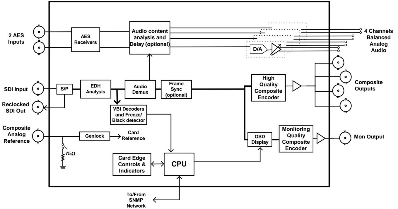
Figure 1-1: 7736CEM-A4 Block Diagram
