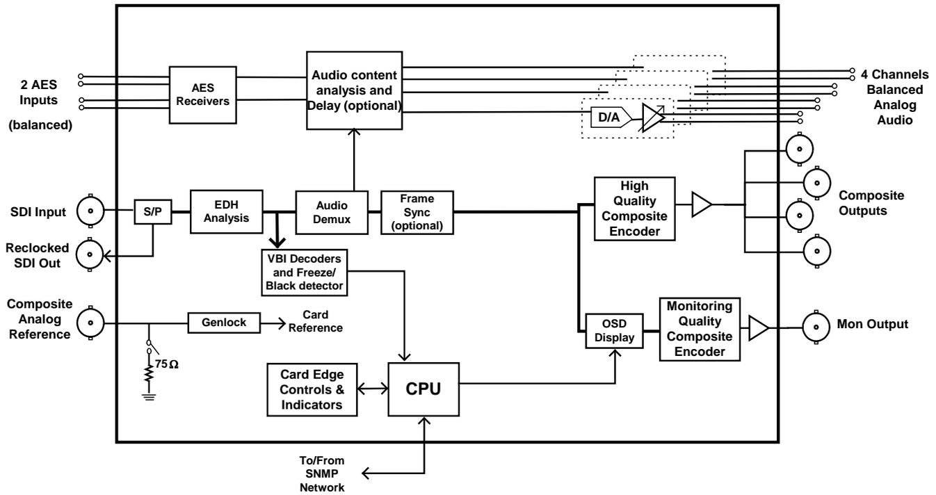
Figure 1-3: 7736CEM-A4-B Block Diagram
