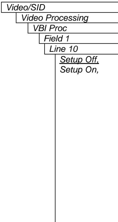
SDI video does NOT have a 7.5IRE pedestal. In NTSC, the VBI lines may or may not have a 7.5 IRE pedestal, depending on the signal present on that line. This control allows you to apply setup on the line, if needed.
