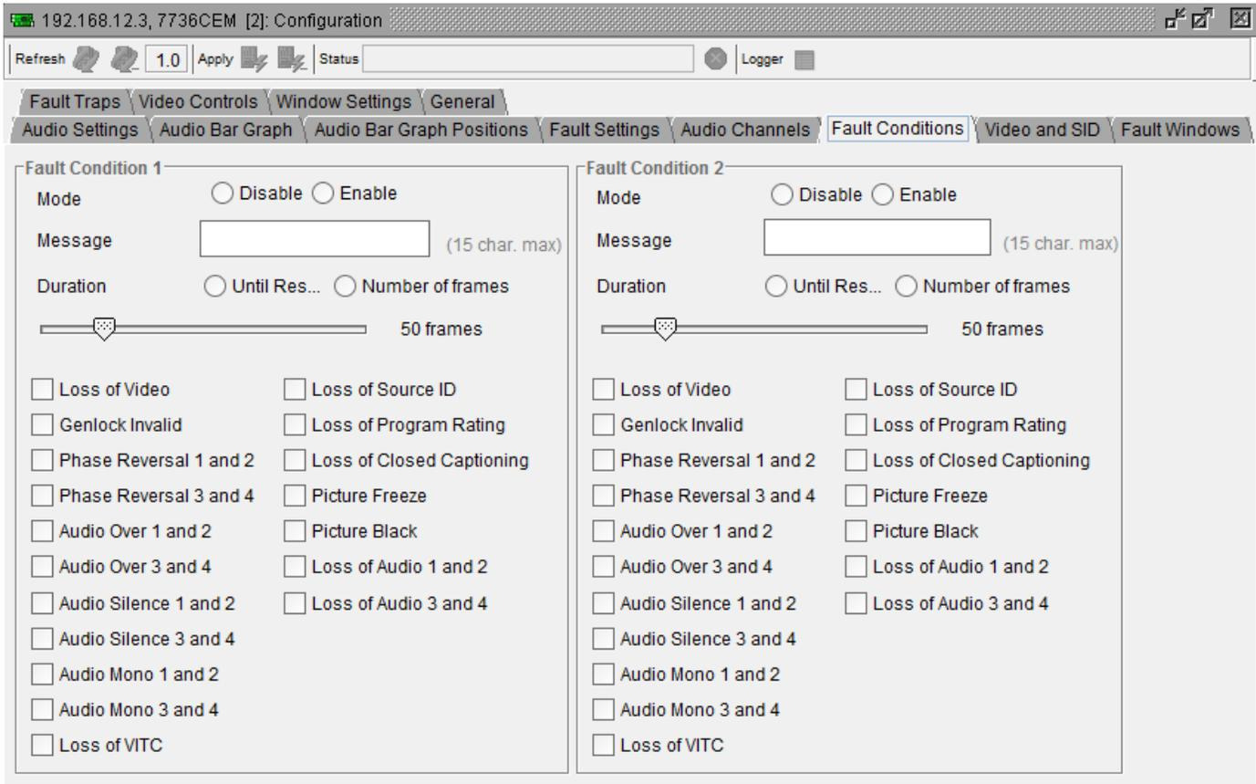
Figure 8-9: Fault Conditions Tab
