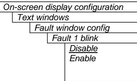
This control determines if the Fault 1 window will blink or be on solid when the fault is active.
