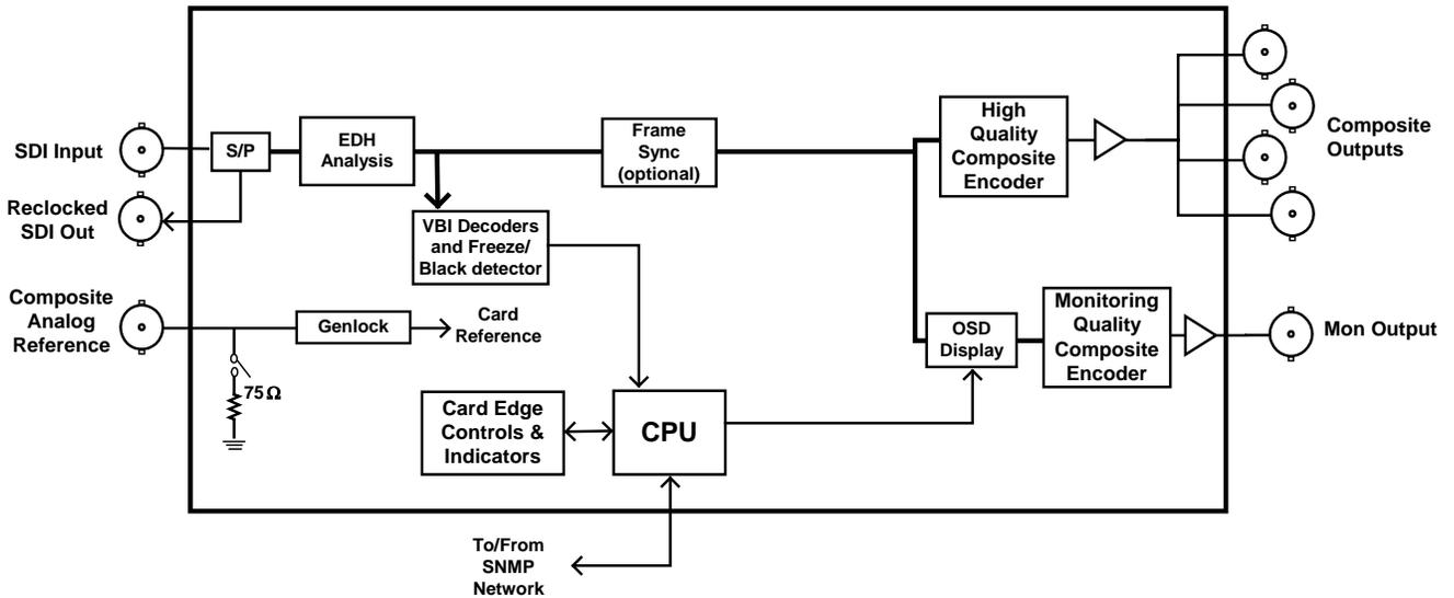
Figure 1-2: 7736CEM Block Diagram
