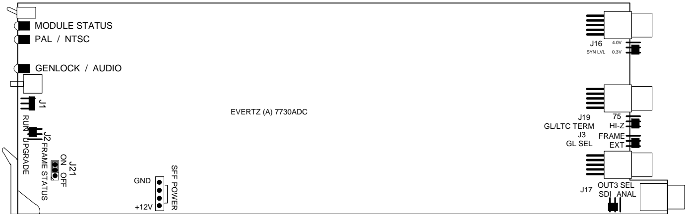
Figure 10-1 : Location of Jumpers on 7730ADC Main Board
