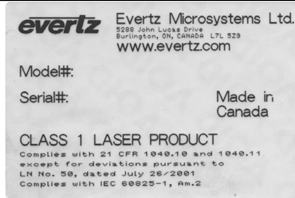
Figure 2-2: Reproduction of Laser Certification and Identification Label
