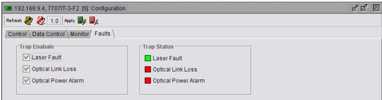
**Figure 7-4: Faults Tab**
