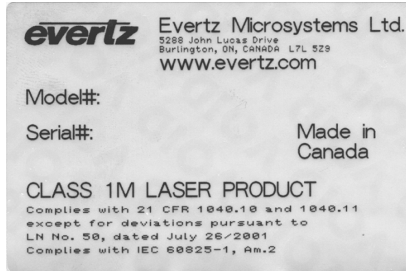
Figure 2-3 Reproduction of 7706LT Certification and Identification Label for Models that are Class 1M Laser Products
