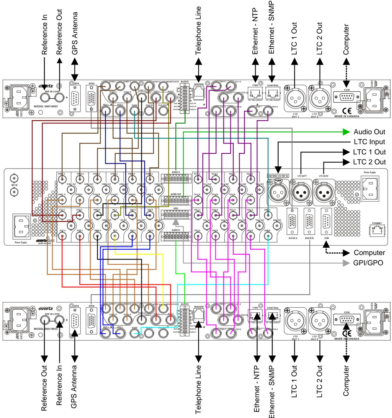
**Figure 2-2: Redundant Master Clock/SPG with Auto Changeover System Diagram**
