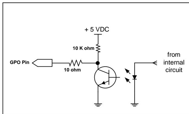
**Figure 2-5: GPO2 Output Circuitry**
