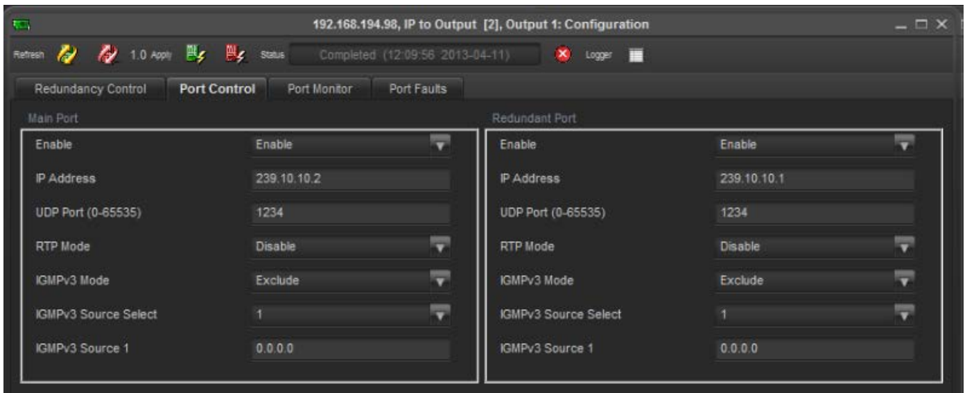
Figure 4-11: IP to Output Port Control
