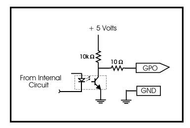
Figure 2-9: GPO Output Circuitry
