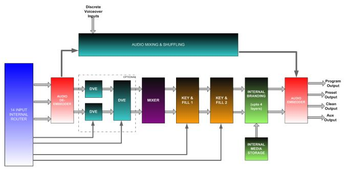
Figure 1-2: 3025SW General Block Diagram
