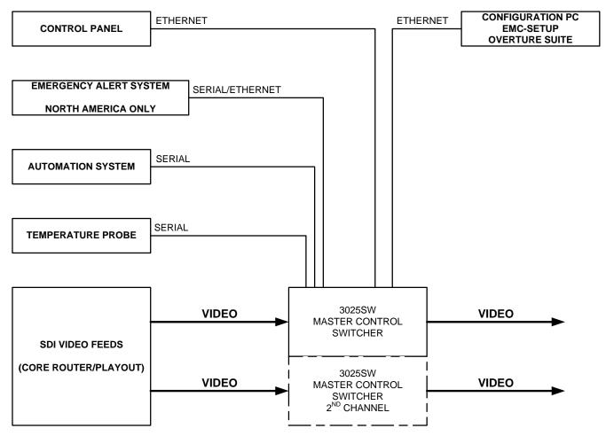
Figure 1-1: 3025SW System Diagram
