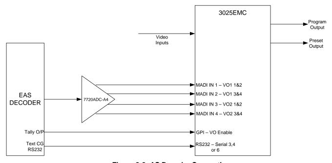
Figure 8-2: AS Decoder Connection
