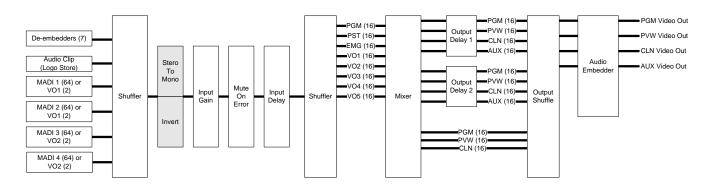
Figure 3-4: Audio Block Diagram
