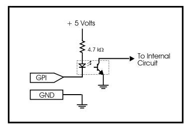
Figure 2-8: GPI Input Circuitry
