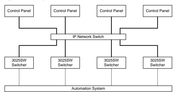
Figure 3-2: 3025EMC Multi-Channel System
