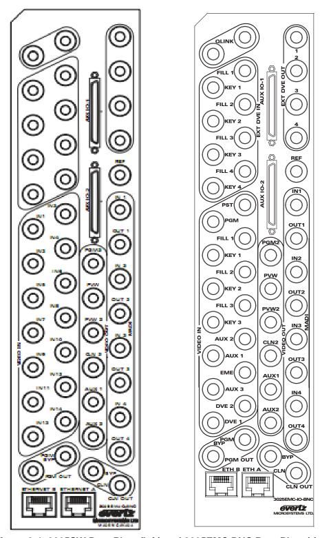
Figure 2-4: 3025SW Rear Plate (left) and 3025EMC BNC Rear Plate (right)
