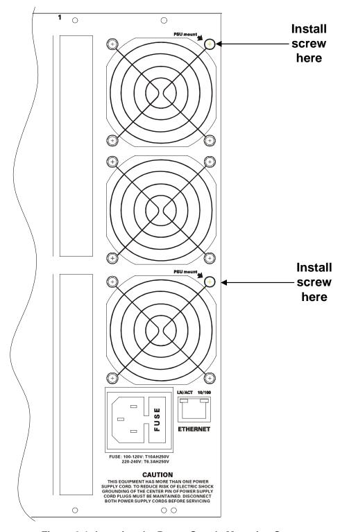
Figure 2-1: Locating the Power Supply Mounting Screw
