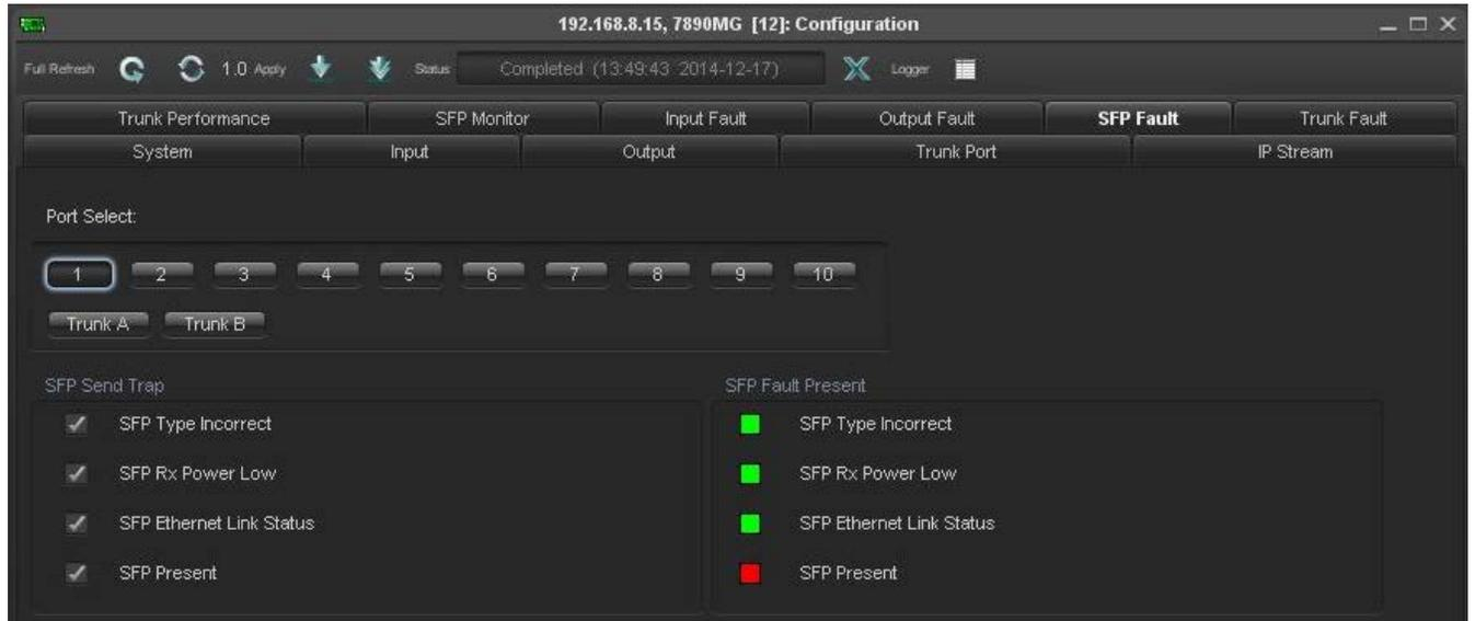
**Figure 4-10: VistaLINK® PRO - SFP Fault Tab**
