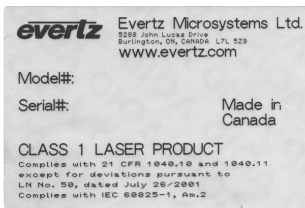
Figure 2-46: Reproduction of Laser Certification and Identification Label
