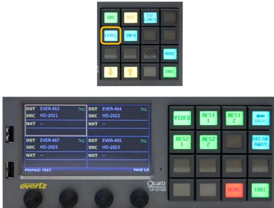
Figure 7-8: Level Button Display
