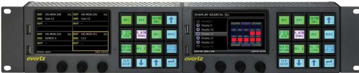
Figure 2-6: Two CP-2116E-H Mounted in a 2RU CPH-RMB
