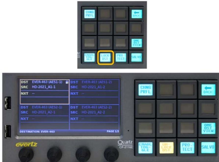
Figure 7-15: Selecting the “LOCK DST” Button
