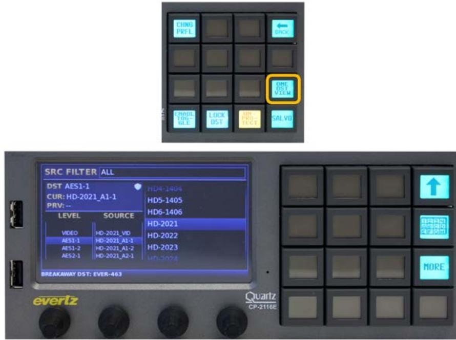
Figure 7-18: Selecting the “ONE DST VIEW” Button
