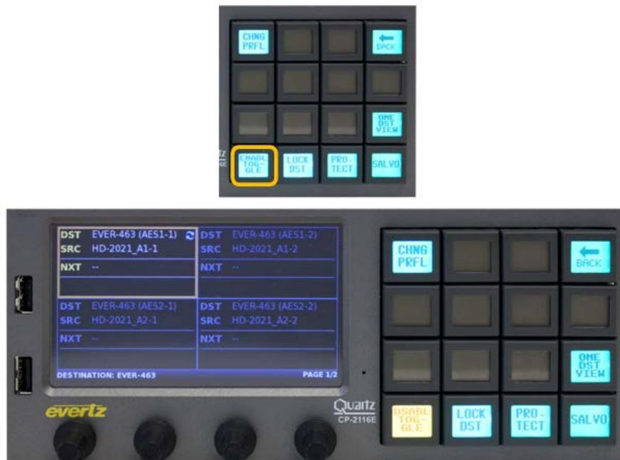
**Figure 7-14: Selecting the “ENABLE TOGGLE” Button**
