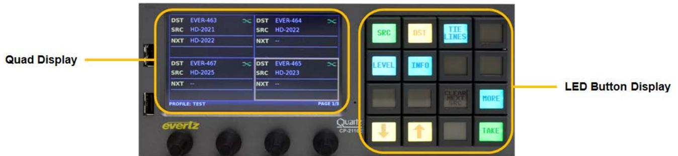
Figure 7-1: Front Panel Display
