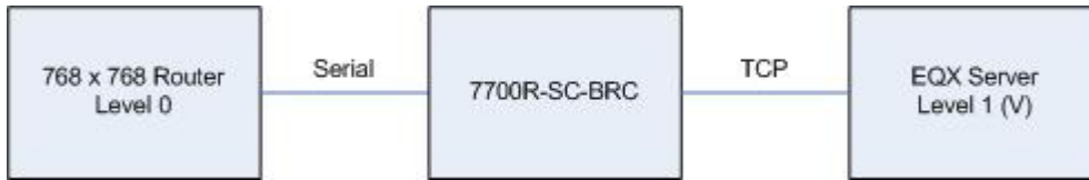
Figure 7-15: Evertz Control NVEP Router Example
