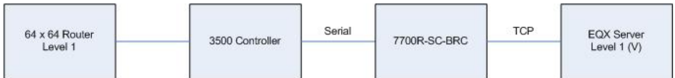
Figure 7-1: CPU Link No. 1 Single Router Example
