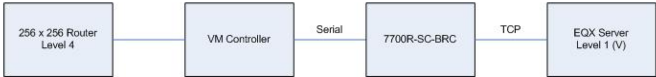
Figure 7-5: Evertz Control VMSI 3000 ASCII Single Router Example
