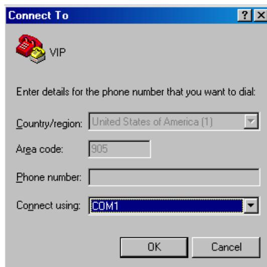
7. Select COM1 for the "Connect using" setting. If COM1 is in use, choose an alternate COM port.
