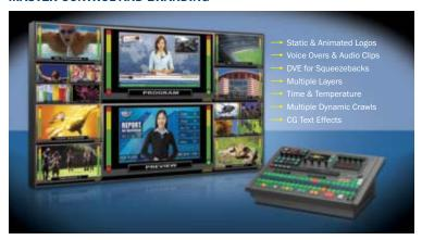
The Company's master control switchers allow users to assemble program streams and insert interstitials such as advertising and promotions for upcoming programs. Switching between the sources (e.g. programming and advertising) allows users to perform voice-overs, wipes, fades, fades to black and a host of other functions.
