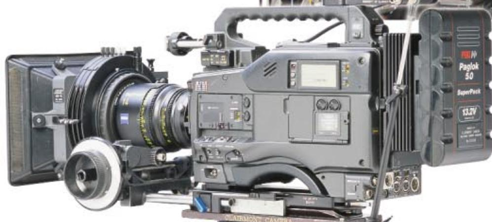
Clairmont's modified F900s have many special features that set them apart from the pack. These include rugged stainless steel B4 lens mounts, repositioned controls, custom carry handles with controls, 12v outlets and Steadicam mounts, and a host of other improvements. They combine the features Cinematographers need with contemporary digital technology.
