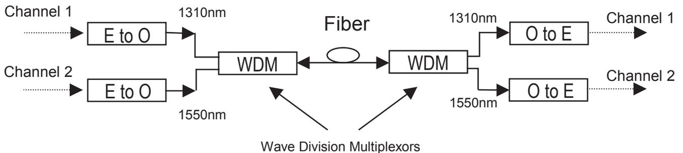
Fig 4. Combining two signals onto one fiber
