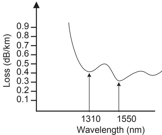
Fig 2. Minimum loss at 1310nm and 1550nm
