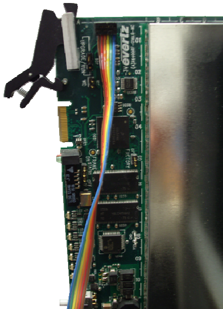
Figure 20 - Output Card Upgrade Header With Upgrade Cable Connected
