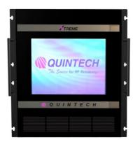
The XTREME-256 matrix is a flexible matrix switch which can be offered as a symmetric 128x128 or asymmetric fan-out 96x160 or 64x192 and fan-in 160x96 or 192x64 in a 12 RU chassis. Designed for high reliability, the matrix provides redundant and hot swappable power supplies, controllers and fans, hot swappable switch cards, and a dedicated redundancy switch path. The matrix also has independently controlled input and output gain/attenuation, allowing signal adjustment for varying cable lengths.
